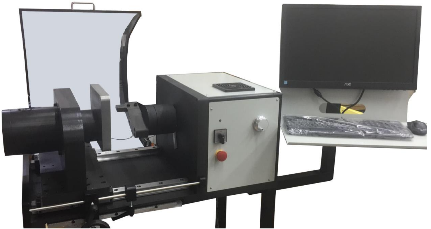
T500 fitted with ARC Spring Testing fixtures
